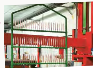
10. Refinar con bronce blanco mediante 25 baños (galvanoplastia) Refinement with white bronze through 25 baths (galvanic)
